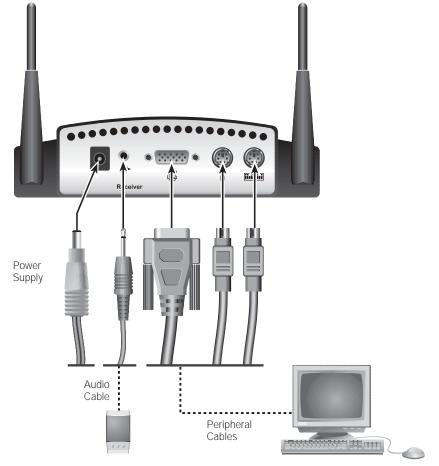
Figure 2.2: LongView Wireless Receiver Installation Example
